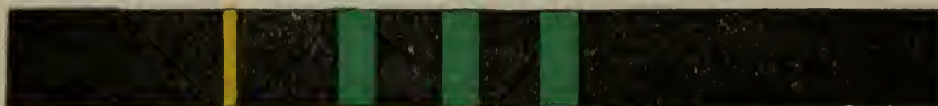
Fig. 14—Spectrum of boracic acid; the yellow is the sodium band always seen.
